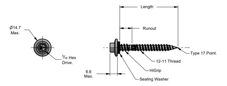
**Note**Lengths from underside of sealing washer and includes compression.
