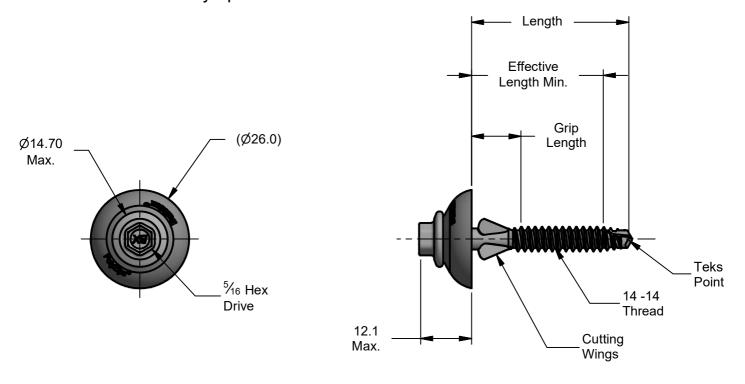
**Note**Lengths from underside of sealing washer and includes compression.
