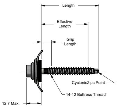
**Note**Lengths from underside of sealing washer and includes compression.
