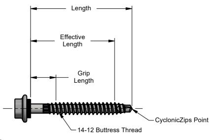
**Note**Lengths from underside of sealing washer and includes compression.
