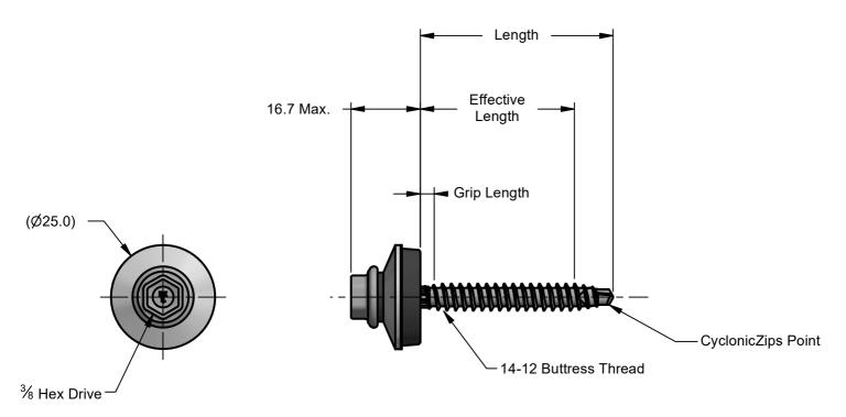
**Note**Lengths from underside of sealing washer and includes compression.
