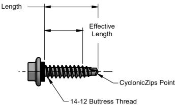
Lengths from underside of sealing washer and includes compression.
