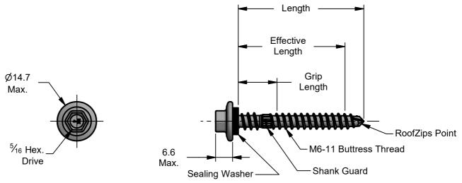
**Note**Lengths from underside of sealing washer and includes compression.
