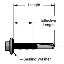
Note Lengths from underside of sealing washer and includes compression.
