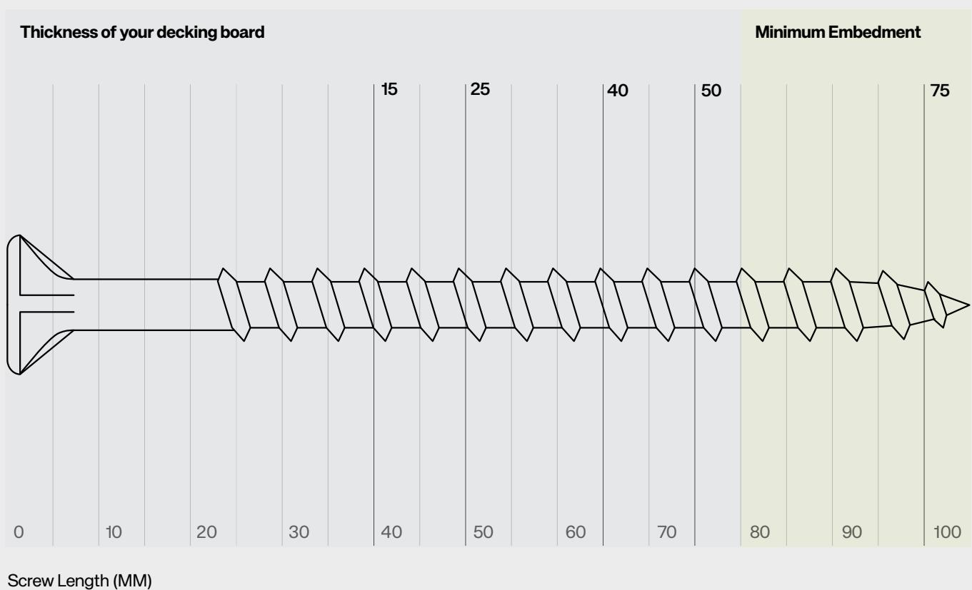
To ensure proper timber-to-timber embedment, the embedment should be at least twice the thickness of the material being fastened. For example, if fastening 20mm decking timbers, a 40mm embedment into the decking frame is required.
